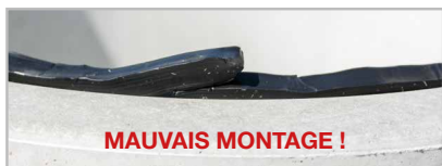
Fermer le joint correctement.
