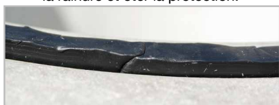
Fermer le joint correctement.
